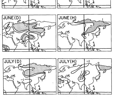
FIG. 6. Normalized difference ( $\Delta$ ) fields between the D and H experiments and the control run for surface temperature for the months of May through July. The regions of stipling or hatching indicate  $\Delta$  values less than -2.0 or greater than 2.0, respectively. See section 2b for the definition of  $\Delta$ .
