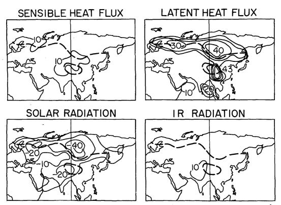
FIG. 16. Components of the surface heat budget for the averaged D experiments minus control for June (W  $m^{-2}$ ). The dashed line is the approximate position of the snow line in the model. Positive/negative values represent fluxes into/out of the earth/ocean surface.
