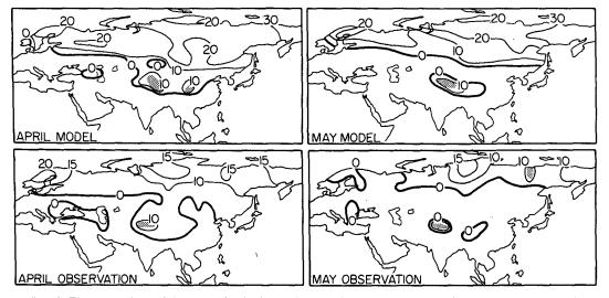
FIG. 2. The comparison of the snow distribution and depth given by the model's climatology with observations. The contours estimate snow depth in centimeters of equivalent water. The heavy solid line indicates the approximate position of the snow line. The stippled areas represent large snow accumulations associated with the Himalayas, etc.
