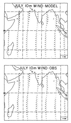
FIG. 4. Comparison of averaged control run July wind velocity with the long term mean obtained from ship reports. The winds are typical of 10-meter anemometer height. The large arrow in the lower right corner of each panel corresponds to an eastward directed wind of 20 m s<sup>-1</sup>. The model winds have been projected onto the 2°  $\times 10^{\circ}$  grid of the observation set. This illustration is courtesy of N. Graham.
